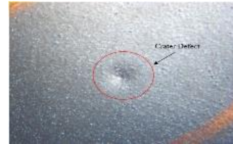
Crater from volatile contaminant
